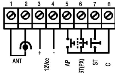
When programmed as a stop or photocell, the configurable input must be NC (negative logic).
